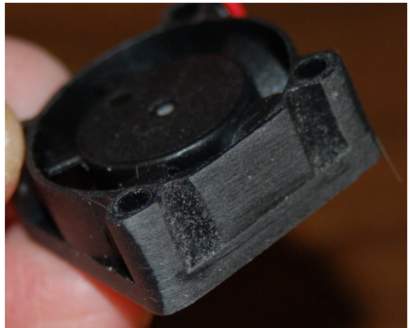
Fig. 3.6-1: Thinning down the fan.
