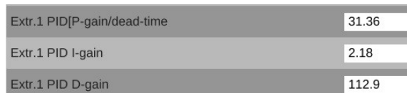
Fig. E-4: Extruder PID settings.
