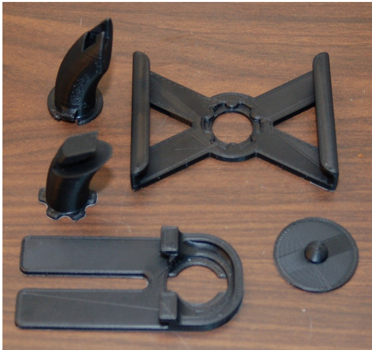
Successfully printed tablet mount components.
